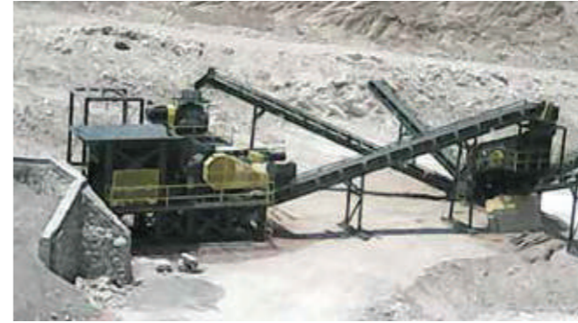
● 100TPH Crushing plant
