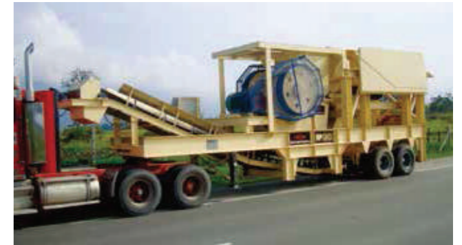
● 100TPH Crushing plant-2
