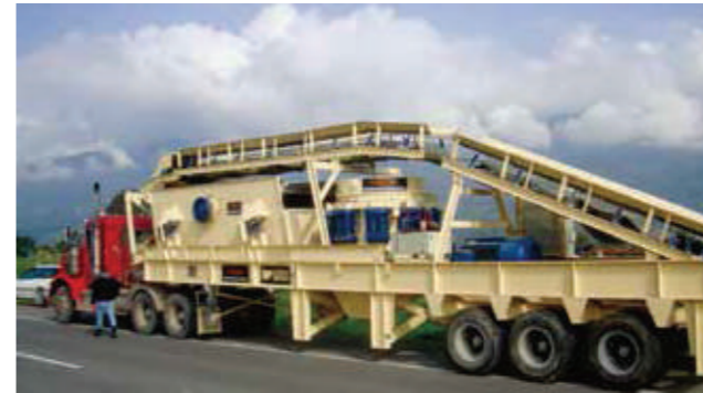
● 100TPH Crushing plant-1
